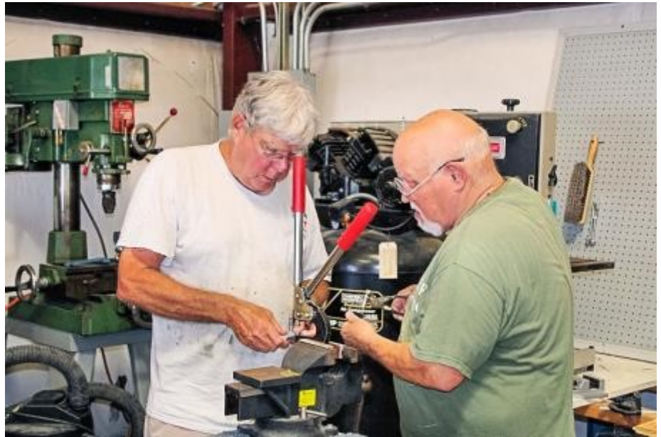
John and Keith setting rivets on the landing light support rib.
