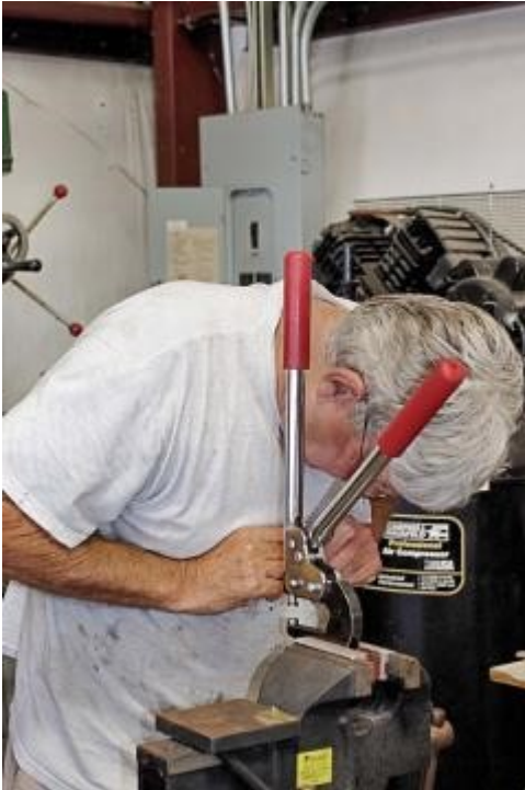
John and Keith setting rivets on the landing light support rib.
