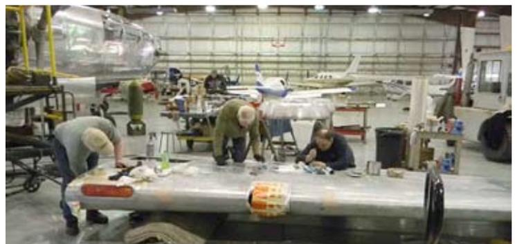
Removed the engines, props and sent them out for over haul and removed all the gear for inspection and repair as necessary.
