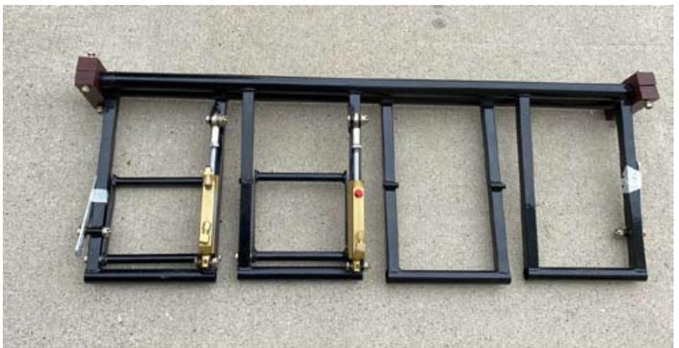
**New Toe Brakes welded up and ready to install. (above)**
