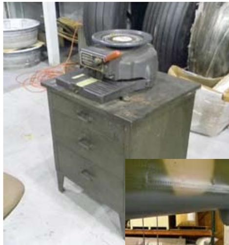
And you ask where did the stencils come from, we made them. The Weeks hangar has a 1940's stencil machine much like the one used in WWII. Here's a pic, fun to do, along with
