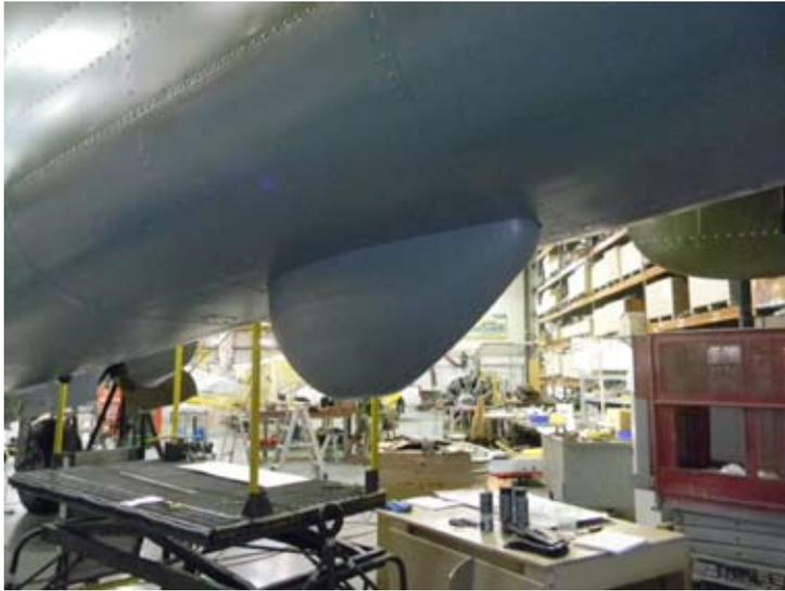
The last picture is the bumper in the back to protect the plane if the pilot over rotates on take off. I was glad to see it installed. I made the metal template during the last trip so they could cut the hole in the bottom of the fuselage to mount this rather large "bumper".
