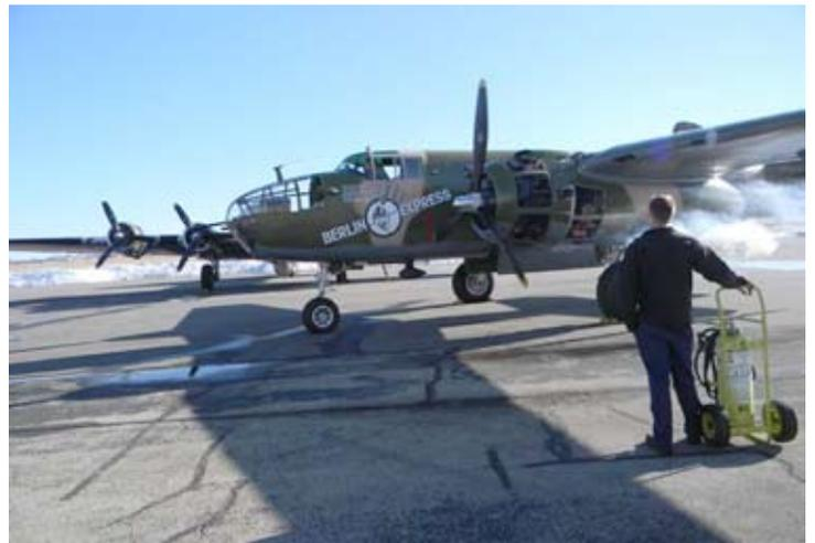
John the lead from the weeks hangar was in the cockpit doing the run up and gave us a down load of how it went. All gauges were working a good first run up. He turned to me and said it was slightly rough on one mag, so would I pull all the plugs and check them. I always wondered what it was
