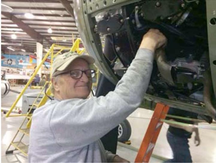
So back out for two engine runs. It turned out the no fuel flow problem was they had not opened the emergency fuel shut off valve for the starboard engine. First to turn the props through. I helped on the port engine and used my shoulder. Not a good idea, I still have a bruise.
