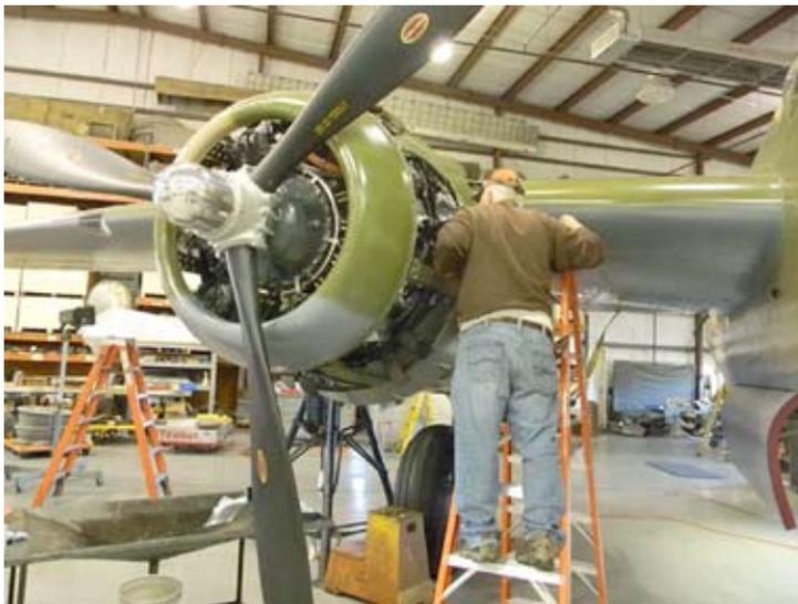
The first engine run was exciting. It definitely was a long awaited event. To start this process while still in the hanger we pumped oil into each engine and checked for leaks and to see if we registered some pressure on the oil pressure gauges. To do this we needed to also turn the engine through. We had done this prior to me putting in the plugs.
