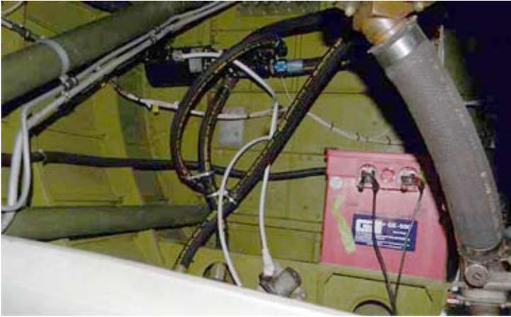
Next was connecting it to a solenoid inside a junction box in the accessory section. From the pic below you can see it was a busy area to work in. The cable is one of the big white ones in the picture. Tidied up some other wires and the project was done.
