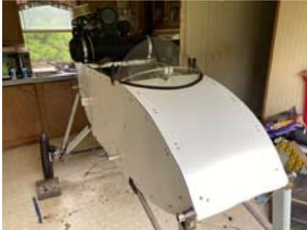
installed (Thanks Ray Robinson), the fuselage has been skinned and has been moved to the garage for center section rigging. As soon as the engine has sufficiently proven itself and the rigging complete, then the outer wing sections will be rigged to the fuselage in the recently prepped hangar at the airstrip.
