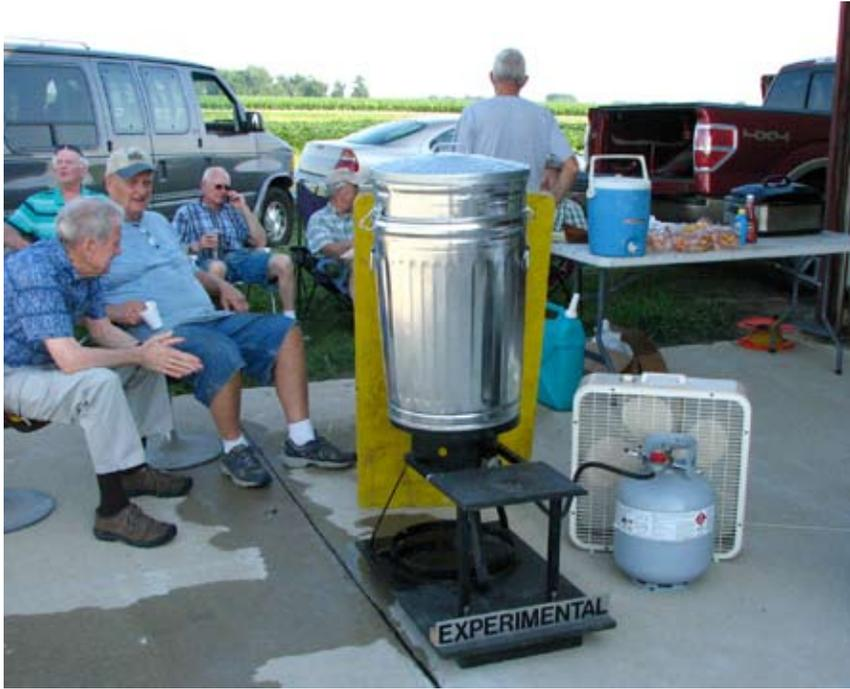
*The corn steamer is made from two garbage cans, one inside the other and powered by a propane burner. Worked pretty well, just took longer than originally predicted.*
