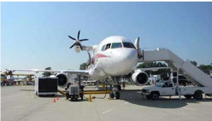
a new special test aircraft with an extra engine;
