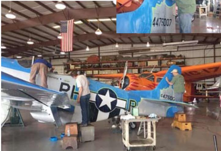
blue for painting. This involved taping off the areas, sanding with 400 grit wet and dry, washing and cleaning the area, covering the rest of the airplane and once painted by EAA personnel we did the clean up. Basically a three day process. Here are some pictures.
