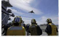
Advanced: The X-47B can reach an altitude of more than 40,000ft, has a range of more than 2,100 nautical miles and can reach high subsonic speeds, claims the navy.
