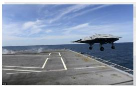
Lift off: The drone takes off from the end of the George H.W. Bush's flight deck. The X-47B is able to operate totally using artificial intelligence in its on-board computers which merely need to be set objectives by the drone's human operators. Critics have warned the technology is a step towards the development of 'killer robots'.
