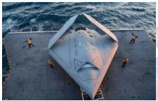
Space saver: The X-47B has a wingspan of more than 62 feet - wider than that of an F/A-18 Super Hornet - so they must be folded up to conserve space at sea
