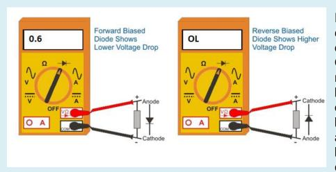
Diode defects can be either open or short. Open diode means diode behaves as an open switch in both reverse and forward-biased conditions. So,
