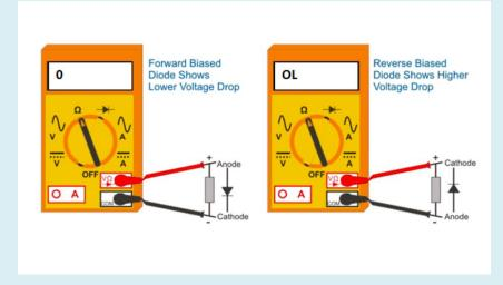
The above figure illustrates a proper working diode, DMM in Resistance (Ohm Mode) shows a very low resistance in the forward-biased condition and a very high resistance or OL in reverse-
