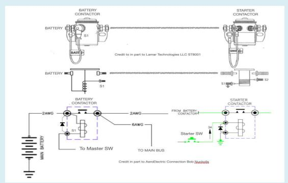
Installation of Catch Diodes on the Battery and Starter Contactor
