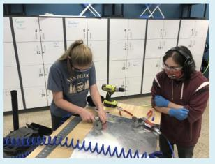
Sixteen very enthusiastic students are actively engaged and learning about riveting and riveting tools. They are discovering 2024 AlClad aluminum and how to cut, debur, layout hole patterns, drill, match drill and rivet universal, flat head rivets,
