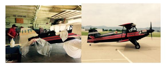
Brian had flown many Skybolts. N193SM is a Skybolt on steroids! Clipped wings, open front passenger seat, closed aft pilot seat with a whopping aerobatic, fuel injected, opposed cylinder, 540 cubic inch, 310 horsepower engine, designated as an AlO540. This monster engine swings a three bladed composite MT constant speed propeller and consumes 14 gallons of fuel per hour at best cruise. All of this with only a 25-gallon fuel tank.
