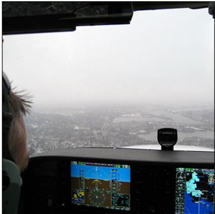
While snow may not be a serious structural icing threat, it can lower flight visibility below VFR minimums within a matter of seconds. Flying through snow can also be quite disorienting to some pilots. Whether you are flying VFR or IFR, be sure to turn on your pitot heat and scan those instruments, especially if you lose sight of the horizon. In this situation, your autopilot may be your best friend.
