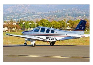
While we taxi, the engine oil is starting to warm up slowly but because the propeller stays in low pitch during this time, the warmer oil does not necessarily circulate to that area.
