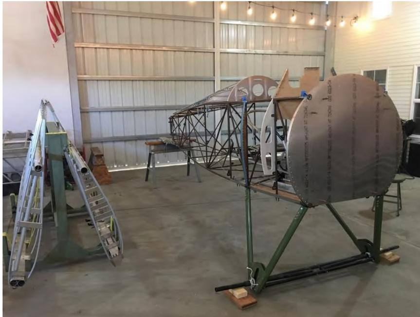
“Wings and tail off so I can build up the fuselage sides. Sides and top are aluminum panels from seat forward.”
