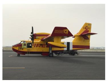
This plane dropped in for fuel on Saturday at Lewiston Airport. New turboprop added for power and efficiency. This plane takes a mile of lake to fill its tank for a fire run. I was parked in the same spot with my Cessna 172 a half hour earlier.
