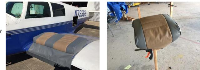
with the elastomeric paint and the seats, photos show the darker grey applied but had some lifting issues when the masking was done for the lighter gray(where the tan still is), paint and seat covers were shipped back to the manufactures lab to resolve the issue. Still has a few things to do yet; repair of the corrosion in the tailcone, landing
