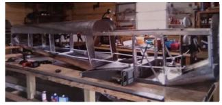
The CX4 is a low wing, single-seat conventional landing gear equipped aircraft although Monte has opted for the nose wheel conversion, which the main gear legs had just came in.
