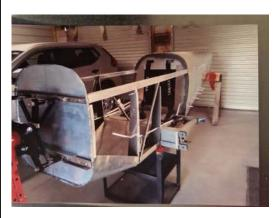
Designed to be simple to build and safe to fly. The name of the plane, CX4, is taken from an old radio show featuring Hop Harrigan, whose plane was called CX4. The aircraft is all metal, 6061-T6 aluminum, except the cowling. The aluminum main gear legs are sourced from a Monnett Sonerai with hydraulic disc toe brakes.
