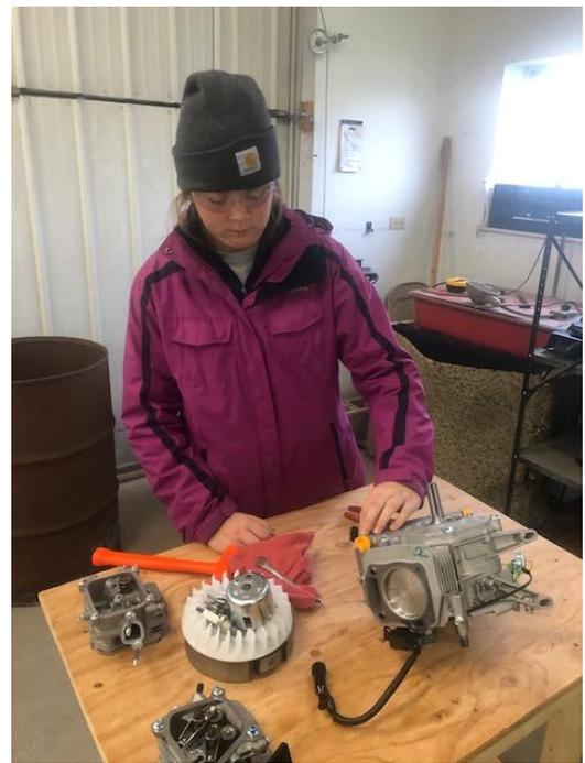
At our last meeting we were also able to get all three engines completely disassembled with the crankshafts, camshafts, connecting rods and pistons completely removed from the engine crankcases. During our December meetings we will begin the process of precision measuring these components to assure their compliance with service wear limits.
