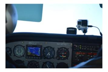
accepted by the FAA in this pioneering effort. In addition to Dynon's proven reliability, the unit delivers a wealth of information to the pilot and even has an integrated angle of attack feature (with the installation of an optional probe). EAA installed the D10A in its 1976 Cessna 172M and submitted to a series of flight tests with an FAA test pilot, which went flawlessly.
