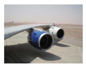
First flown in February of this year, we have completed 125 hours of flight testing with 2 development versions of the Trent XWB. Testing to date has been very successful, and it was time to stress the engine to the upper limit of external temperature. The current mid-day temperature in Al Ain, United Arab Emirates, is 44C, or about 112F. Combined with low humidity, it was exactly the environment we were searching for.
