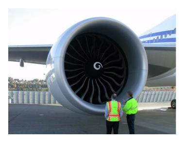
GE90-115B (115,000 lbs thrust) engine with 3D aerodynamics in the carbon fiber fan blades.
