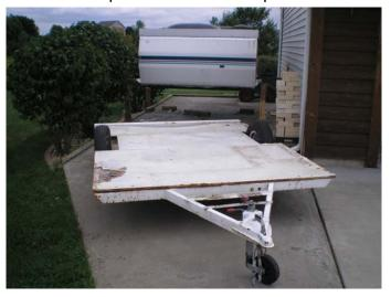
The floor was really soft and in terrible shape so I have gotten to this stage so far. The frame is going to a sandblaster shop for cleaning and
