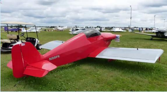
Corey lives in Stillwater, is an engineer with Boston Scientific, and previously worked for Rockwell Collins and Garmin, where he was on 'Team X' which developed the G3X for the experimental market. The Sonerai was designed by John Monet, who also designed the Sonex, as a VW engine powered racer. The Sonerai has aluminum wings but rag on tube for the fuselage and empennage. Corey
