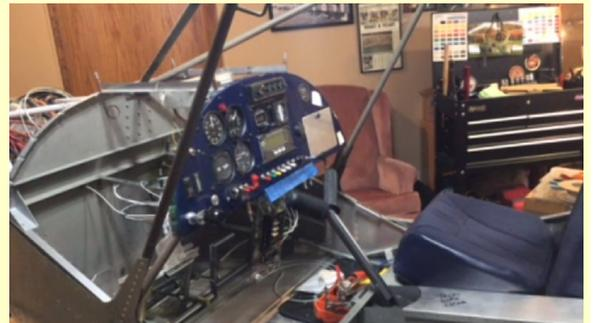
Ed has installed a 120hp Jabiru 3300 six cylinder engine with a Bing Carburetor.
