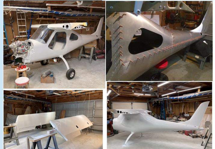
The Merlin is from a Czech company with beautiful and precise predrilling for rivets – he found only 2 holes out of 3500 that needed redrilling. The airframe kit runs \$18k, and the firewall forward kit is \$8k for the 60 hp HKS which is expected to give ~2.5gph eco cruise at 100mph, with a 120mph max cruise, running from a 6 gallon tank in each wing.
