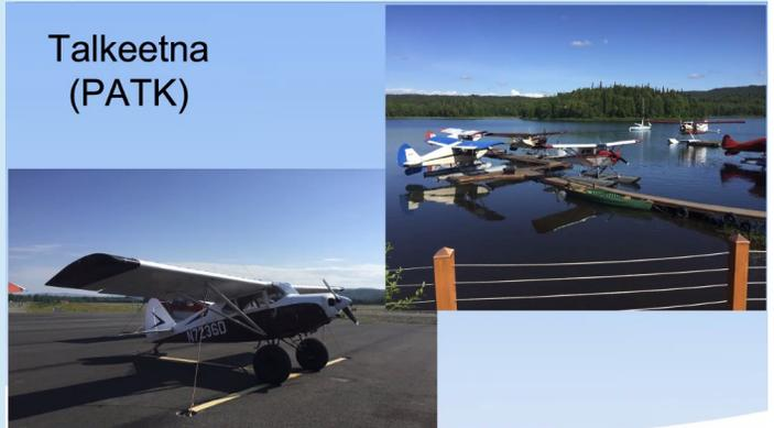
At Talkeetna Laura trained in a Piper Pacer with Tundra tires, practicing gravel strip landing, gravel bar landing, and avoiding gravel damage to the propeller and aircraft. She learned lighter colored gravel bar is dryer, and to overfly to check out, a second time to skim with wheels to feel firmness, to land the third time. During this time she
