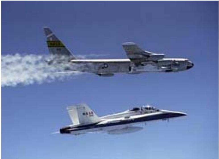
NASA's B-52B launch aircraft cruises to a test range over the Pacific Ocean carrying the X-43 on March 27.
