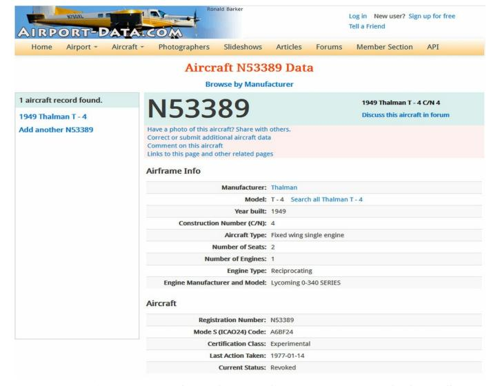
**T-4** 1953 = 4pChwM rg (manual); 135 hp Lycoming O-290; span: 40'0" load: 1050# v: 175/155/45 range: 700. All-wood geodetic construction. [N53389]. Later converted to T-tail with 170 hp O-340. Price FREE.
