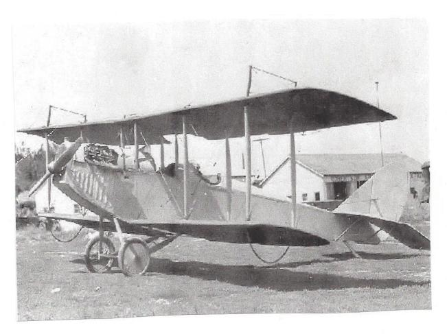
Curtis JN4-D, cost to government in 1917, \$8160.00 Wing span upper- 43 ft. 8 in. lower 33 ft. 11 in. Length- 27 ft. 4 in. Max Wt. 1920 Lbs. Max speed- 75 MPH. Engine- Curtis OX-5, liquid cooled, 90 BHP.
