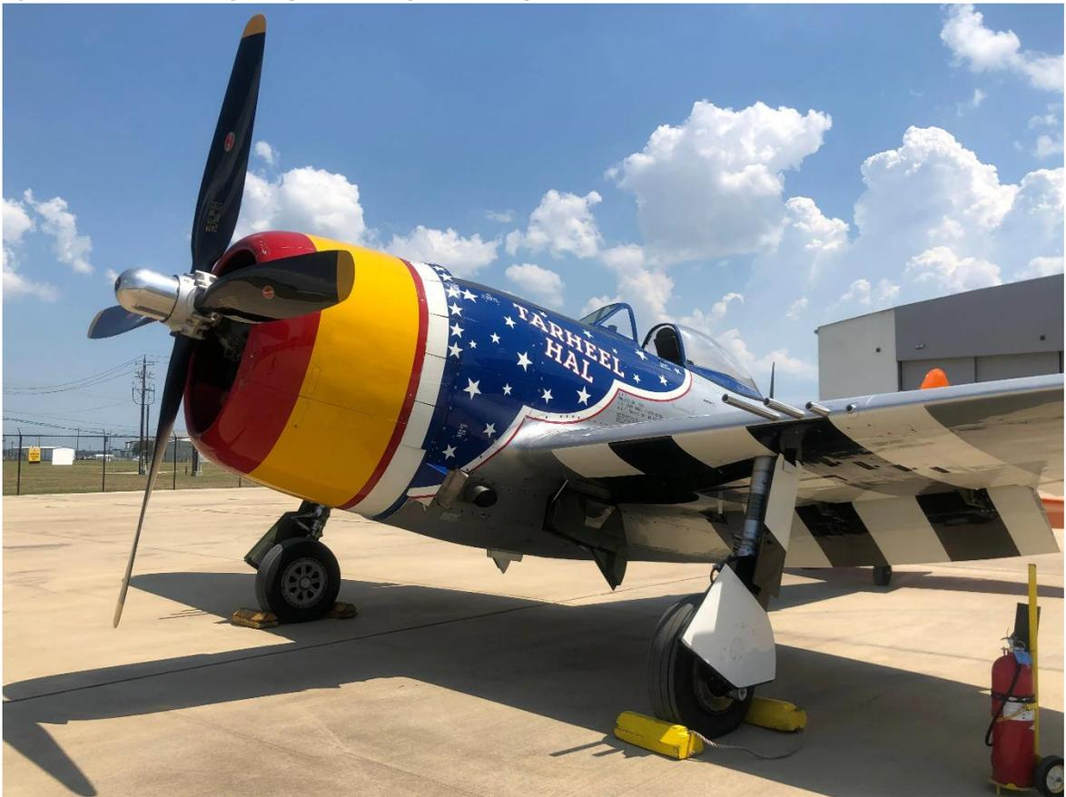
The top speed was 553 MPH with a range of 800 miles wingspan was 41 feet and they weighed 10,000 #'s First flight was May 6<sup>th</sup> 1941 This was a very competitive aircraft great in air combat and devastating in ground support. With her 8 fifty cal. Machine guns you could add 6 more rockets!
