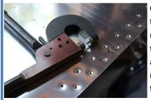
On the thicker materials, such as the spars, the holes need to be counter sunk to the correct depth determined by the thickness of the dimpled material being riveted on. There are three different thicknesses of the aluminum wing skins, so three different depths to the more than 1,500 holes.
