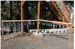
the main wing spars, labeled with wire tags so they find their way back to the correct spot, grease and ink marks cleaned off and finally spray primed with a self-etching primer. This step also includes the interior part of the wing skins.
