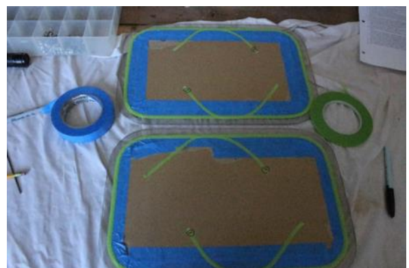
SKYLIGHT CLECOED IN PLACE WITH SPECIAL ADJUSTABLE CLECOS AND THE MULTI-LAYERED TAPING
