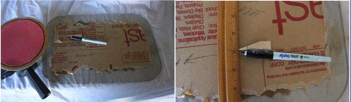
TOOLS FOR FITTING A WINDOWS: 4 ½" GRINDER AND FINE-POINT PEN FITTED WITH A SPACER FOR EXACT FIT
