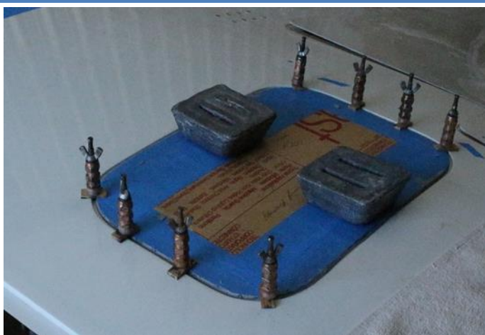
SKYLIGHT CLECOED AND WIGHTED IN PLACE
