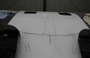
For a change, the elevator tip fairings fit properly and are nearly done. Just waiting on some ordered nut plates to complete the installation.
