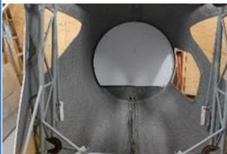
The main bulkhead behind the baggage area has an open center to facilitate access but needs a cover piece for structure. The plans called for a thin sheet aluminum cover with materials supplied in the kit. I cut it out and with lots of effort, bending, stretching, standing on my head, etc. got the attaching nut plates installed. It seemed a little flimsy and prone to oil-canning so with leftover Cozy foam, fiberglass and epoxy, I made a fiber-
