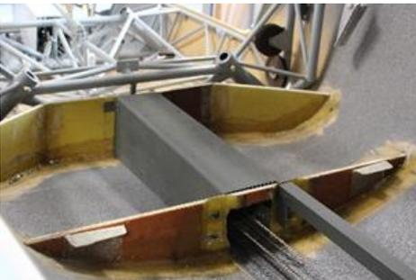
from the plans, you automatically double, triple or quadruple the time for project completion, but it was a fun exercise and I think it came out looking good. I glassed quarter-inch-foam-sandwich support bulkheads and used quarter-inch oak plywood covers to fabricate a fixed cover on the aft half and two hinged door covers on the forward section.
