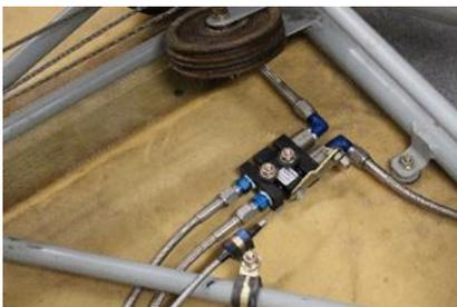
I purchased braded brake lines to replace the supplied Nylaflo lines that are prone to breakage, and installed them with the optional parking brake. The other two planes I have built lacked a parking brake and created a challenge when parking on a slope without someone to insert or remove the wheel chocks.
