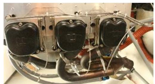
I fabricated the oil cooler hoses and installed them between the engine oil filter and the remote oil cooler.
