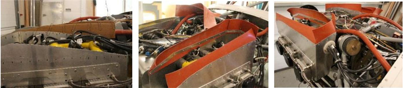
The last project of the month was installing a cabin heater muff on the exhaust pipe and routing a hose to the firewall valve. The muff consists of a shroud around a portion of the exhaust pipe that has a stretched spring wound around it to increase surface area. There is an outside air source hoses to the muff inlet. The air is heated through the muff and exits to the firewall mounted cabin heat/defrost/bypass valve.
