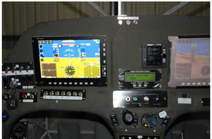
Good news – the com radio/intercom, Bluetooth ADS-B receiver/AHRS system, engine instrument system, auxiliary fuel tank pump timers, and EFIS are mostly debugged and working. Added a resistor to the fuel pressure sensor and rewired a GPS input to the EFIS. The Mode S/ ADS-B TailBeacon X transmitter is not working and will need to be sent in for repairs (bought used, “working when removed”).
