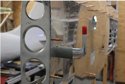
Then all the holes in the upper and lower main spars and several ribs are enlarged from #40 to #30.
