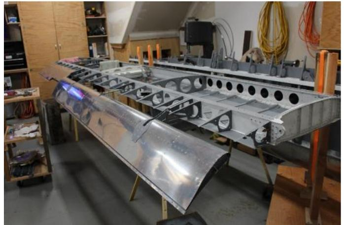
The 15 gallon main and 10 gallon auxiliary fuel tanks were installed. The auxiliary fuel tank fuel is pumped to the main tank so a fuel pump complicates the plumbing system. Also, many builders recommended positioning the fuel pump in a different place than in the plans in order to have better access for inspection and maintenance. Anytime you deviate from the plans, even following someone else's directions, adds hours to the build.
