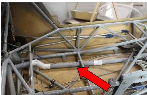
I installed a PVC conduit under the seats to the aircraft front for all the wires to the aft fuselage. These include the magnetometer, electric elevator trim and position sensor wires, and wires for the uAvionix tailBeacon X.
