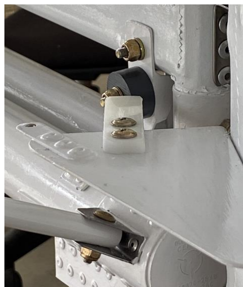
Left PVC Rudder Stop is engaged
