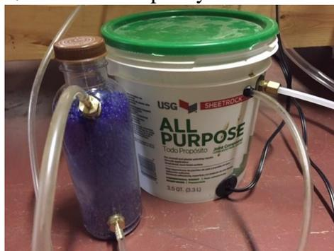
After writing this, I decided to change the configuration of the system. I now am using a small spackle container only for the pump, the drink bottle is now free standing next to the spackle container, this way I can easily see the condition of the desiccant. Maybe I will build a support that holds both the container and the bottle. If I keep writing this and keep thinking about it, I may be making more mods. For now, it is running 24/7.
