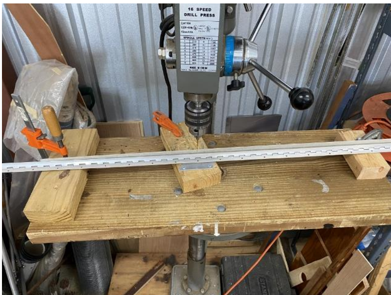
Hinge Leaf Bending Jig using Vise-Grips.
