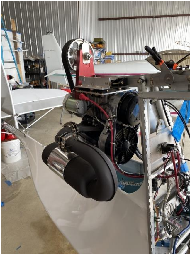
Rotax 503 mounted on the root tube at the firewall
