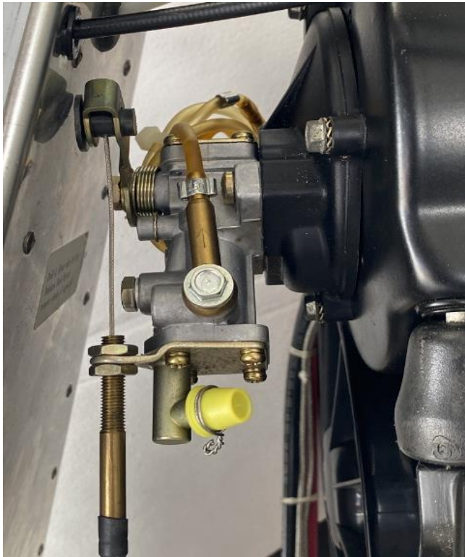
Third cable from the throttle splitter connected to the oil injector pump.
