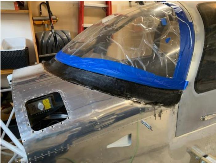
I moved the primary voltage regulator from behind the sub panel in the middle bay to this location. I was looking in this access hole recently and realized I had the perfect location to install the voltage regulator right here. Easy access for future maintenance.
