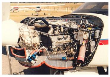
Two ignition systems: Electronic control and trigger.
