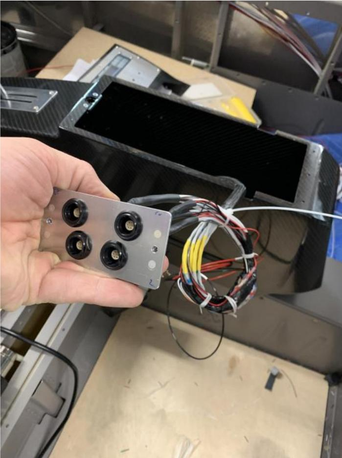
Following the footsteps of a couple others who have gone before me I attached the silver relay housing to the SDS CNC'd ECU enclosure. The wiring harness for the two just seemed to be made for this.
