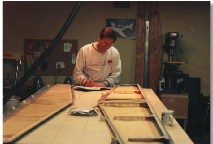
Greg Kessel Checks the Horizontal Stabilizer Pre-closing
