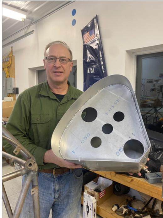
Tyler Mullen visited us during his Spring Break from Purdue. He dove right in and tied down the aluminum base on the turtledeck for the headrest fairing. We started a several week process of hand-priming the rear fuselage to prevent any more surface rusting. Longerons for the sides of the fuselage are being measured for new aluminum ones to replace the original wooden ones.
