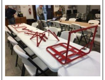
The big news on the metal front is that everything EXCEPT the fuselage has been primed and/or painted. Primed but unpainted pieces (tail feathers and landing gear) will be covered in fabric. The struts, the seat and control stick, the engine mount, and other parts of the landing gear are all now shiny RED!
