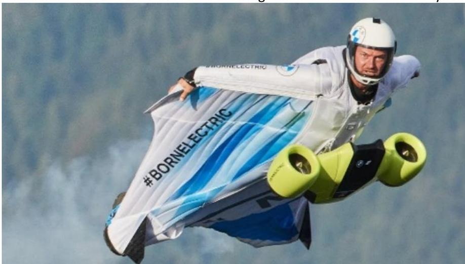
*Editor Comment – The unit comprises two encased carbon impellers that spin at 25,000 rpm producing about 20 HP. I wonder if they could attach wheels on the unit with a nose gear on his helmet. It would be an exciting landing*
