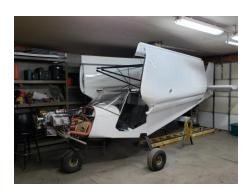
Getting a lot closer to firewalling the throttle. The wings are installed and fold nicely. The engine is installed but still working on the cooling plenums. Almost done wiring and getting all the instruments installed.
