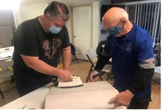
David Yegge and Rod Beckwith III heat shrinking the Poly Fiber material around the airfoil with the "Magic Weapon" .....
